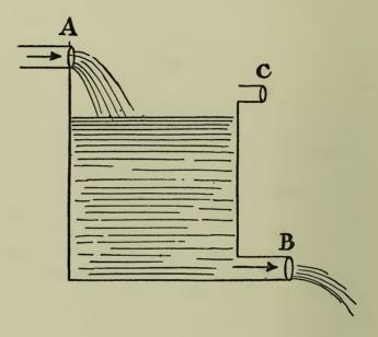
Imagine an open vessel, filled nearly to the brim with water. It has an escape pipe B, through which the water constantly flows out, while an equal quantity flows in at the supply pipe A. Thus the surface of the water always remains at the same height. If the conditions are altered and the vessel overflows, this may be due to several things.
